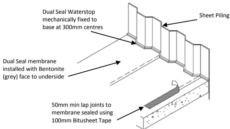
Dual Seal Membrane installation to sheet piling. Dual Seal installed with Bentonite (grey) face to underside
